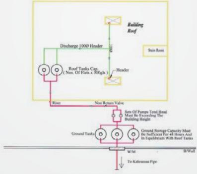
Multistory Building With Two Header Installation Of Individual Water Meters On Each Floor ( Drg. No. : 2 )
